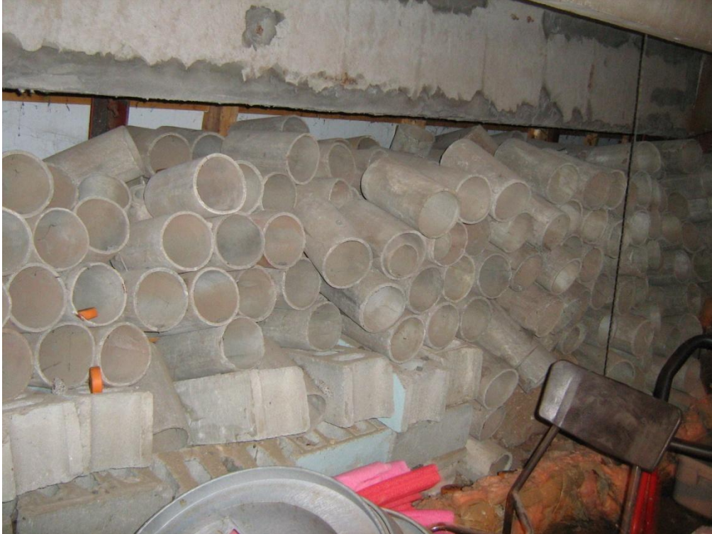
Photo 3: Stored ACM Transite pipe sections, (Rm. 33). 1952 era underseat crawlspace.
